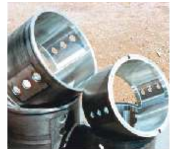
White metal bearings repaired
