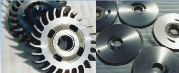
Vacuum pump spares reconditioned with HP/HVOF coatings and tig welding.
