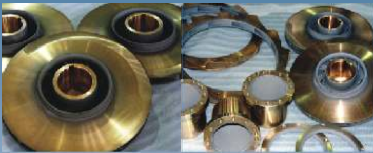
Pump impellers are sprayed with tungsten-carbide to increase life expectancy.
