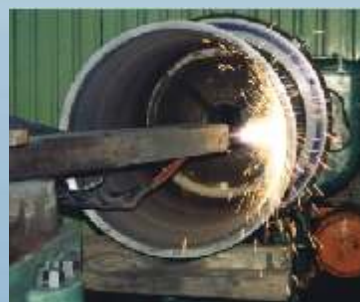
Bore sprayed with 420 s/steel and machined.
