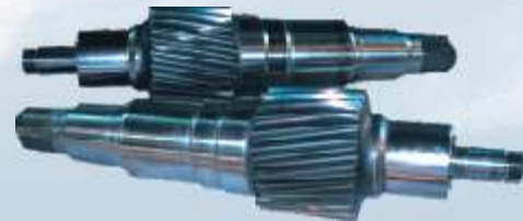
Pinion shafts repaired with micro submerged welding
