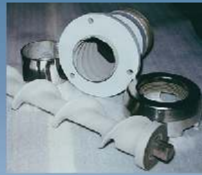
Plastic manufacturing plant, parts are coated with a HP/HVOF coating to extend life (also used in the food processing industry)
