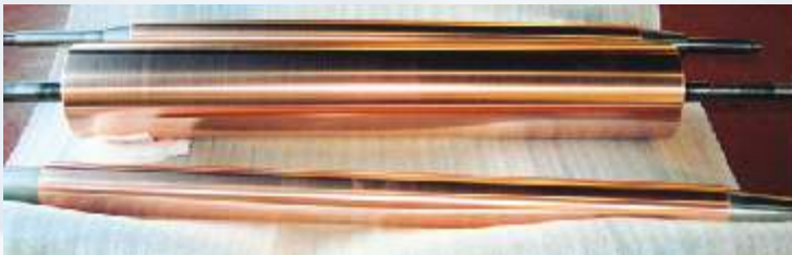
Copper printing rolls repaired.
