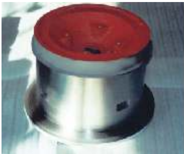
Wire drawing blocks repaired
