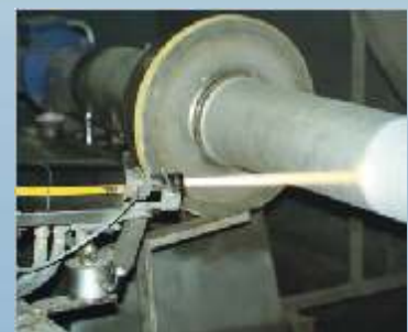
HP-HVOF coating of plunger
